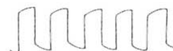
(c) Capacitance excessive
